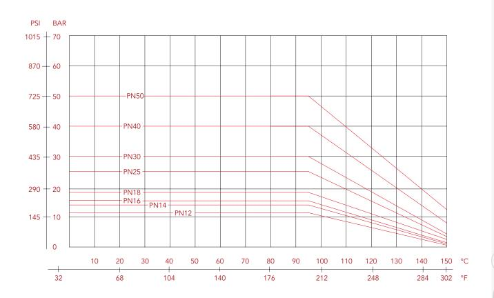
The values shown by the dropping lines state the maximum limit of employment of the valves. The shown valves are approximate.
